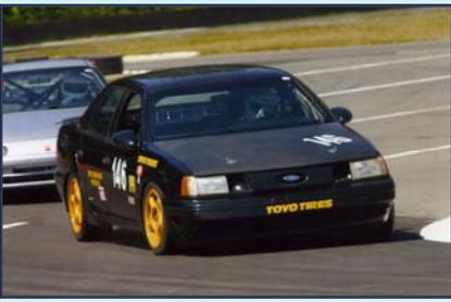
Les's current car, the 1990 Ford Taurus SHO (Super High Output) 3.0 liter DOHC Yamaha V6, 5 speed trans 240 HP @ 3000 lbs is pictured in the photo above. Les built the car himself featuring suspension modifications, racing tires, shocks and brakes for maximum cornering speeds, full roll cage and all safety equipment to meet regulations.
