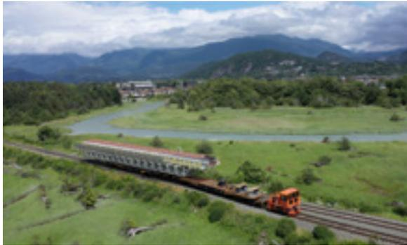
offsite laydown area for major capital equipment and offsite construction. The 3.8 km rail line connecting the BCRP site to SQT allowed for massive oversized modules and capital equipment to be moved to SQT, loaded to barge and transported to Neptune Terminals for installation. This solution avoided all use of roadways and bridges and offered a safe, economic and environmentally responsible way to move the equipment.
